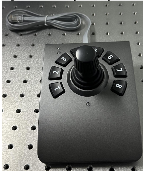
Fig.13 The external displacement stage control rocker can be adjusted in 8 levels of accuracy.
